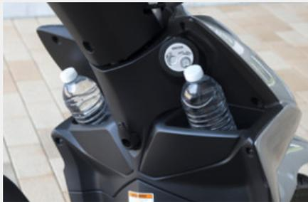
Both left (600 ml) and right (500 ml) storage compartments provide ample room together with covered key functionality layout above the right pocket.
