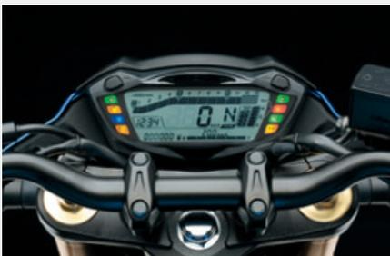
The GSX-S750 features a lightweight, brightness-adjustable LCD instrument panel. Readouts include the speedometer, tachometer, traction control mode status, gear position, odometer, dual tripmeters, coolant temperatures, driving range, fuel consumption, and a clock. You can personalise the tachometer readout from a choice of five display patterns.
