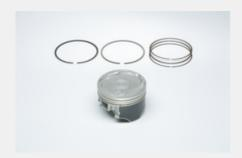
One of the upgraded features in the 645cm3 unit are the resin-coated pistons which is a coating technology to decrease friction in the cylinder, resulting in improved fuel economy and corresponding to latest emission control. Special L-shaped piston rings are also installed for enhanced sealing performance and blow-by gas reduction, all resulting in meeting up-to-date regulations while improving the output and the ease of use.
