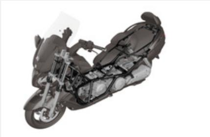
A tubular frame and aluminium-alloy swingarm position the engine and transmission for balance and agility. The frame inherits the long, 1,595mm wheelbase of earlier Burgmans for a sporty, controllable ride and has a newly designed, slimmer tail section for sleeker, sportier bodywork. Plenty of wheel travel (110mm at the front and 100mm at the rear) helps to keep the ride smooth.
