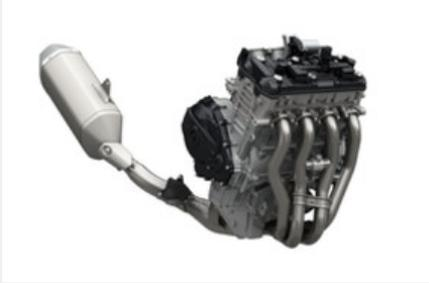
The all-new, 999.8cm<sup>3</sup> in-line four cylinder, DOHC, liquid-cooled engine, is the most powerful, hardest accelerating, cleanest running GSX-R engine ever built. Producing 148.6kW (202ps) @13,200rpm with 117.6Nm of torque @10,800rpm, the new engine surpasses the competition. The design target was simple "Increase top end power without sacrificing low and mid range output" to achieve this Suzuki engineers had to employ advanced MotoGP derived technologies known as the Broad Power System.
