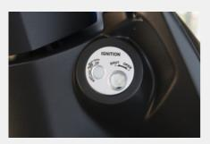
Key hole is covered by lid to prevent motorcycle theft. Easily access the under-seat compartment using the main ignition keyhole, eliminating the need to remove key to open seat compartment.
